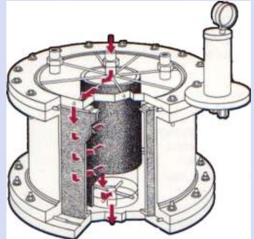
Superflo® columns are based on radial flow chromatography. The columns have three annular channels. The outer and inner channels have equal cross-sectional areas and conduct the fluid flow to the outlet. The middle channel contains the chromatographic packing. Due to the large cross-sectional area of the outer channels and the low bed depth, Superflo® columns allow extremely high flow rates with very little pressure drop.
